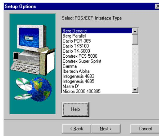
2. When prompted, select the appropriate **POS/ECR Interface Type** for the sales terminal. This determines which driver file is loaded to the ECUs for communication with the sales terminal. (Click **Help** for a description of each type.)
